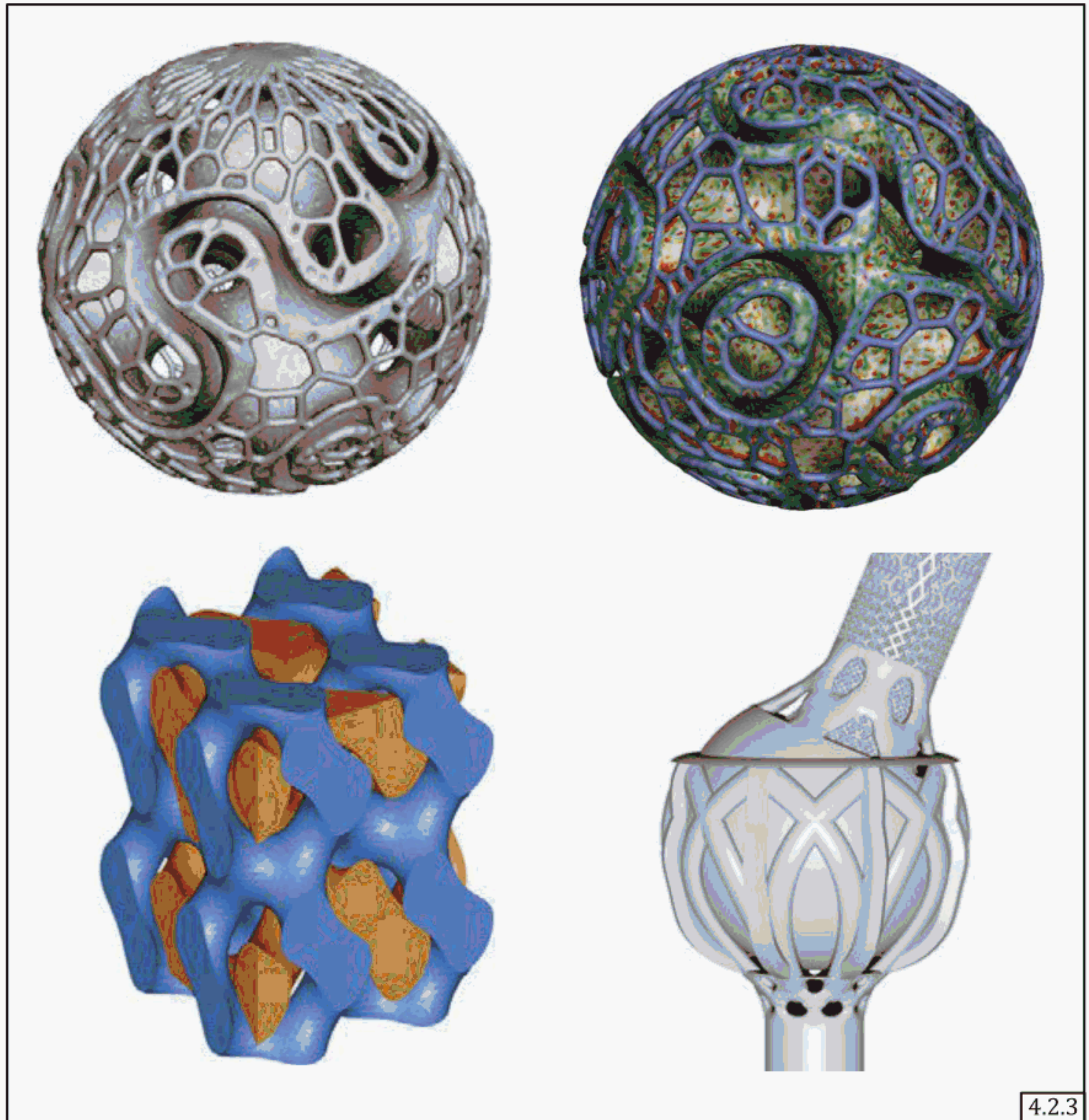
Figure 4-14 Complex Geometries Generated From Topology Optimization
