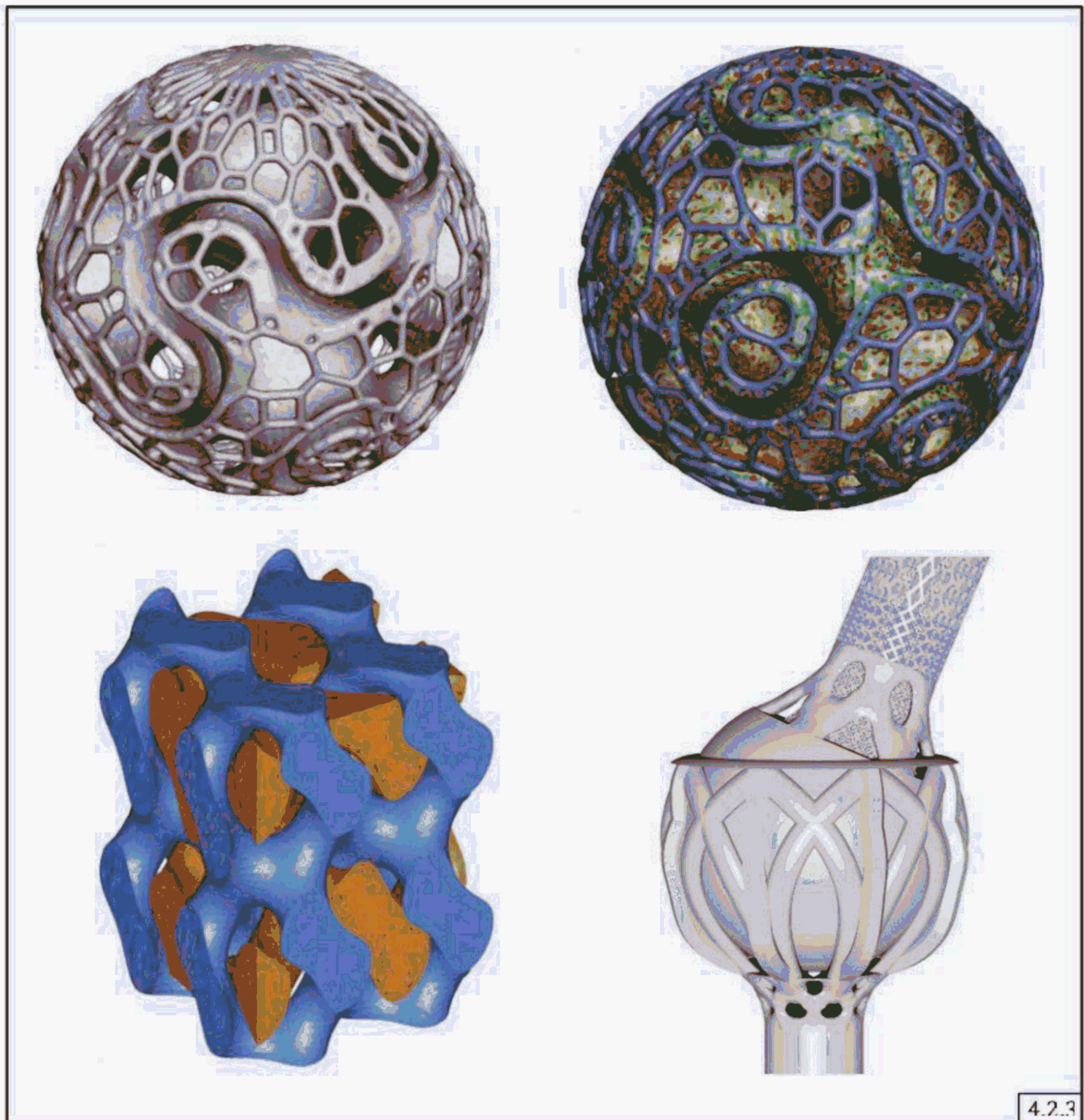
Figure 4-14 Complex Geometries Generated From Topology Optimization
