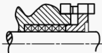
P1: Soft packing without lantern ring
