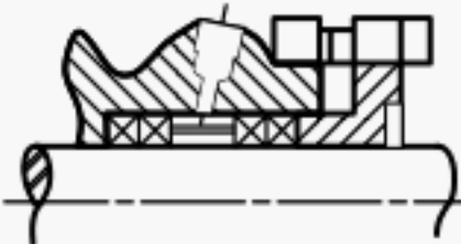
P2: Soft packing with lantern ring. Used for injection or circulation of liquid for sealing, buffering, cooling, etc.
