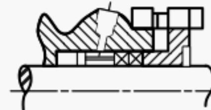
P3: Soft packing with extended flushing throat bushing used for injection or circulation of liquid for cooling, to clear deposits, etc.
