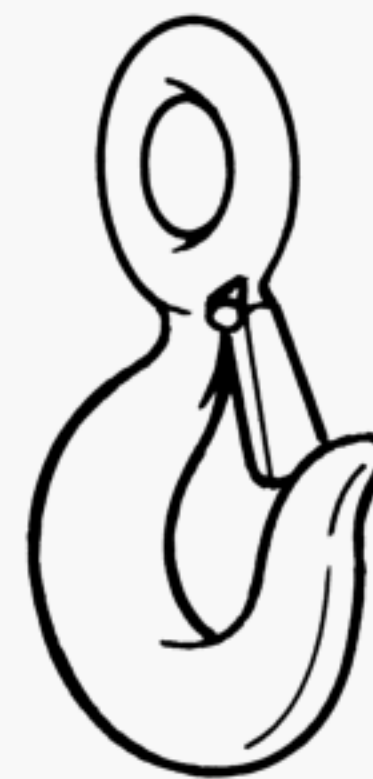
Fig. 12 Self-Closing Flipper Latch (Eye Hook)
