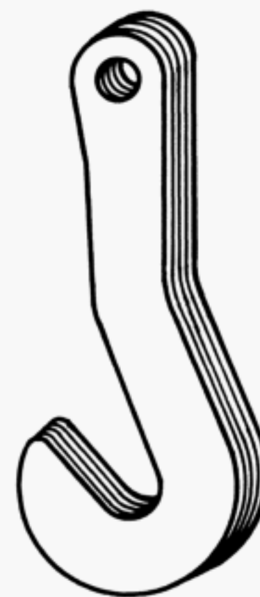
Fig. 16 Laminated Plate Hook
