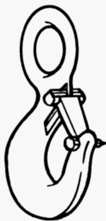
Fig. 14 Self-Closing Tiplock Latch (Eye Hook)
