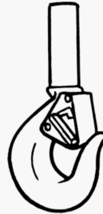
Fig. 10 Self-Closing Flapper Latch (Shank Hook)
