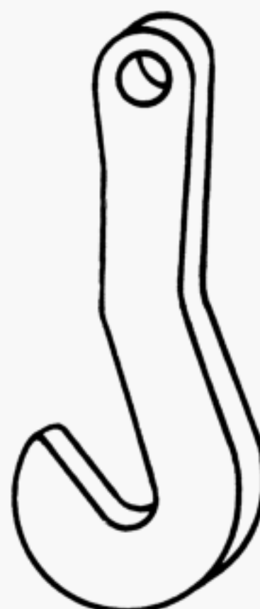
Fig. 15 Single Plate Hook
