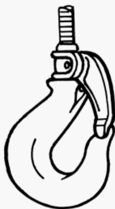
Fig. 9 Self-Closing Gate Latch (Shank Hook)
