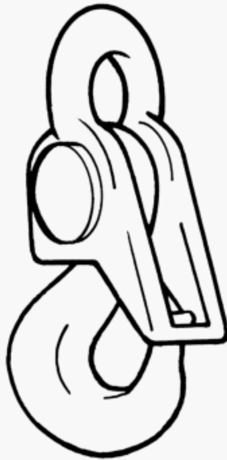
Fig. 8 Self-Closing Bail (Eye Hook)
