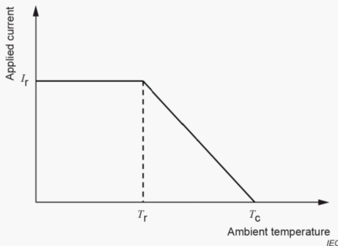
**Figure 1 – Relation between ambient temperature and applied current**
