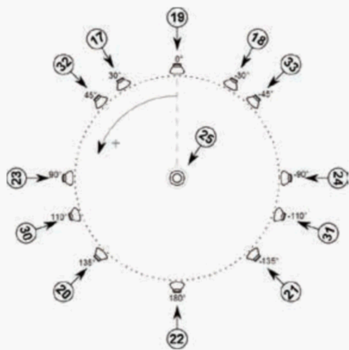
Figure 10 — Loudspeaker positions, upper layer [index 25 indicates the loudspeaker directly above the listener, sometimes referred to as the “voice of god (VoG)” loudspeaker]
